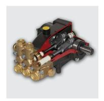
The U-Seals provide better run-dry protection, extend pump life, and allow for inlet water of up to 145°F. Kärcher K3 pumps provide a stronger crankcase with thicker mounting feet and extra-large European made tapered roller bearings for longer pump life. The crankcase is reinforced and comes with the new O-ring seal for leak-free operation. Specially die cast connecting rods provide for quieter operation and longer pump life.
