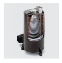
Kärcher's proprietary heating coil is unequaled in the industry for its high heating performance, compact design, and super-efficiency. Double-wall construction — with air passing between the two walls — provides insulation as well as oxygen for the combustion process.
