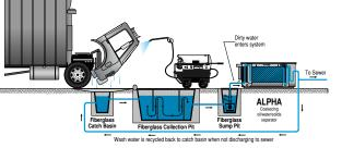
The Alpha can work in conjunction with below-ground catch basins and collection pits or as a stand-alone oil-water separator.
