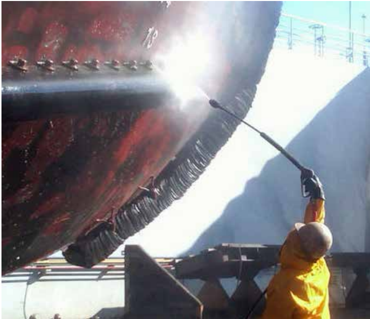
Cleaning a ship's hull is only one of the many applications for the MPE high-pressure washers with cleaning power of 5.0 GPM and 5000 PSI.
