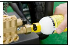
Turn lever to open the valve on bottle
