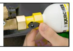
Pull starter cord until fluid begins to exit water outlet. (Do NOT start engine)
